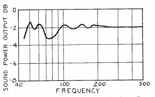
Fig. 4—Power output characteristic of a horn (horn of Fig. 5B. with all dimensions multiplied by 2½) coupled to a 10½ inch, 10 gram, diaphragm driven by a 5 gram aluminum voice coil in a field of 20000 gausses. Damped resistance of voice coil 20 ohms. Impedance of vacuum tube 35 ohms.
