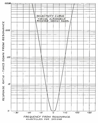
Fig. 10-Selectivity curve-modern automobile receiver.
