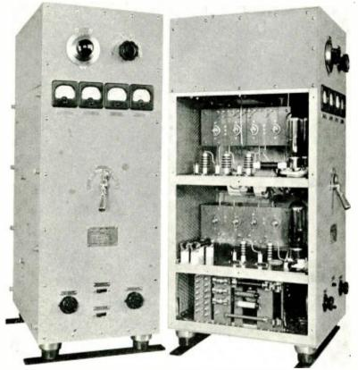
Fig. 1—300-Watt radiotelegraph transmitter.
