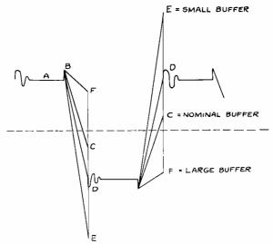
Fig. 6-Vibrator transformer primary wave form.
