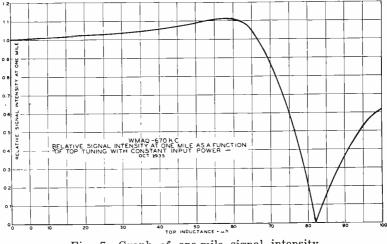
Fig. 7-Graph of one-mile signal intensity.
