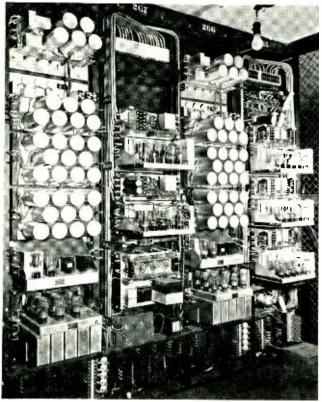
Fig. 7-Synchronizing generators and associated equipment.
