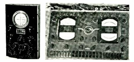
Typical modern servicing equipment. The cathode-ray oscilloscope is also invaluable as a visual aid in school laboratories.
