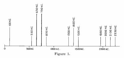
new frequencies made by the rectifier are multiples of the fundamental, that is the second harmonic, third harmonic, etc. of the signal frequency. Where two strong signals exist, a number of cross modulation combinations take place. Let us call the frequency of one of the strong stations a, and that of the other b, then the rectifier generates the following frequencies:
