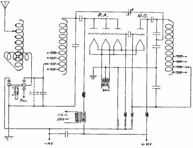
Fig. 4--Schematic circuit diagram of the transmitter.
