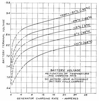
Fig. 7—Variation in battery voltage with charging rate at various battery temperatures.
