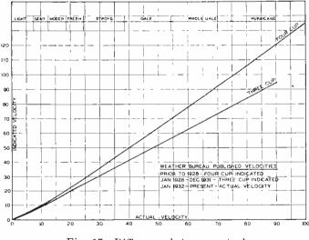
Fig. 17—Difference between actual and indicated wind velocities.
